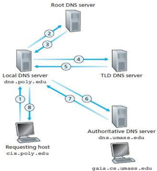
Here DNS query is sent to local DNS server then to root server, then to TLD server and finally to authoritative DNS server. DNS response arrives in the reverse order.
