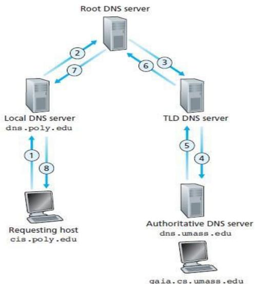
Here DNS query will be sent to Local DNS server, then to root server. Root server sends the IP address of TLD server. Now local DNS server sends query to TLD DNS server. TLD DNS server sends the IP address of authoritative DNS server to local DNS server. Now Local DNS server sends query to authoritative DNS server. Authoritative DNS server sends the IP address of host to local DNS server. Local DNS server sends it to the host.
