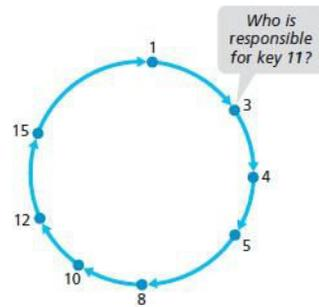
Each peer is only aware of its immediate successor and predecessor; for example, peer 5 knows the IP address and identifier for peers 8 and 4 but does not necessarily know anything about any other peers that may be in the DHT.
