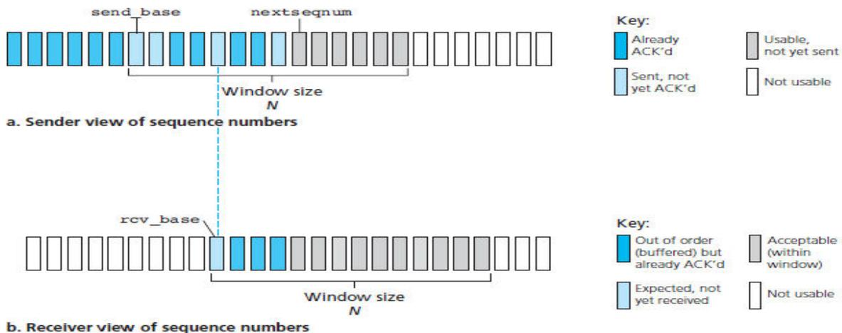
1. *Data received from above.* When data is received from above, the SR sender checks the next available sequence number for the packet. If the sequence number is within the sender’s window, the data is packetized and sent; otherwise it is either buffered or returned to the upper layer for later transmission, as in GBN.
