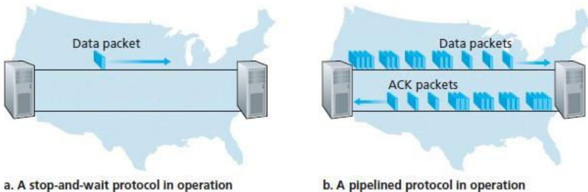
Above Figure (a) shows that with our stop-and-wait protocol, if the sender begins sending the packet at  $t = 0$ , then at  $t = L/R = 8$  microseconds, the last bit enters the channel at the sender side. The packet then makes its 15-msec cross-country journey, with the last bit of the packet emerging at the receiver at  $t = RTT/2 + L/R = \mathbf{15.008 \text{ msec}}$ .
